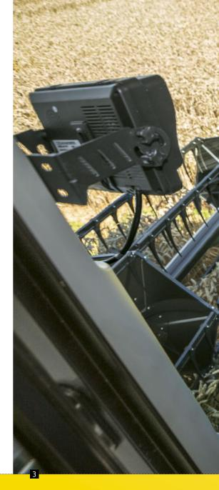
**Corner-post mounted display** Perfectly positioned to avoid interference with your view to the header
