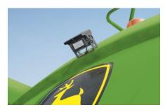
Optional cameras help to observe the rear of the combine during reversing or check chopping distribution. On the unloading auger they help to see inside the trailer while mounted next to the hitch they assist in connecting the header trailer. A separate monitor is mounted in the cab to display the camera picture.
